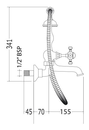
Note: The rear inlets to this Wall mounted BSM model are adjustable to accomodate pipe centres 210-150mm
