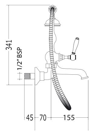
Note: The rear inlets to this Wall mounted BSM model are adjustable to accommodate pipe centres 210-150mm
