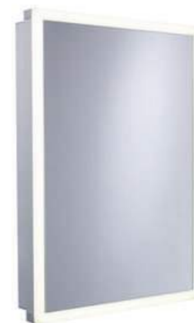
Nook Single Door Cabinet with Integrated LED Lighting Aluminium 500(w) x 700(h) x 117(d)mm 47mm depth when recessed. Fits recess 460(w) x 660mm(h) NO50ALC £640.00
