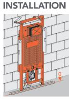
1. Position and level the frame, mark the holes.
