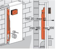
4. Connect to in/out water pipes, put on blind covers and fix the WC.
