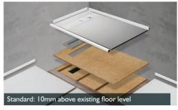
Flooring removed to size of aqua4ma Shower Deck, create a false floor at joist level, add plywood panel to lift shower deck 10mm above existing floor level to allow joining to aqua4ma Floor Panels. Then use aqua4ma 10 mm Panels to waterproof all or part of the floor to the same height as the shower deck.
