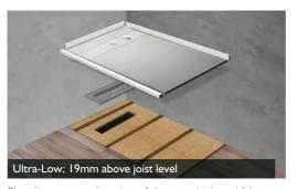
Flooring removed to size of shower deck and false floor created at joist level.
