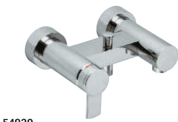
54920 Single lever bath tub mixer exposed, ceramic cartridge with temperature limiter, with automatic return bath tub/shower
