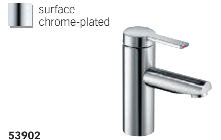
surface chrome-plated 53902 Single lever basin mixer PLAN blue with/without pop-up waste, 1-hole installation, ceramic cartridge with temperature limiter, flow rate limited to 6 l/min.
