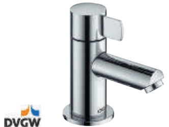
DVGW 54908 Pillar tap without pop-up waste, 1-hole installation, 90° head part with ceramic sealing gaskets
