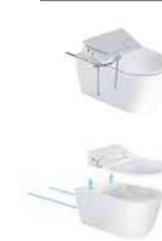
Duravit's patented Durafix attachment system is quick and easy to install. It is invisible, too – the water and electric connections are concealed within the ceramic. The water and electricity connections run through the ceramic without being seen. (Below) An in-line heater heats the water as and when required, and only in the necessary quantity.
