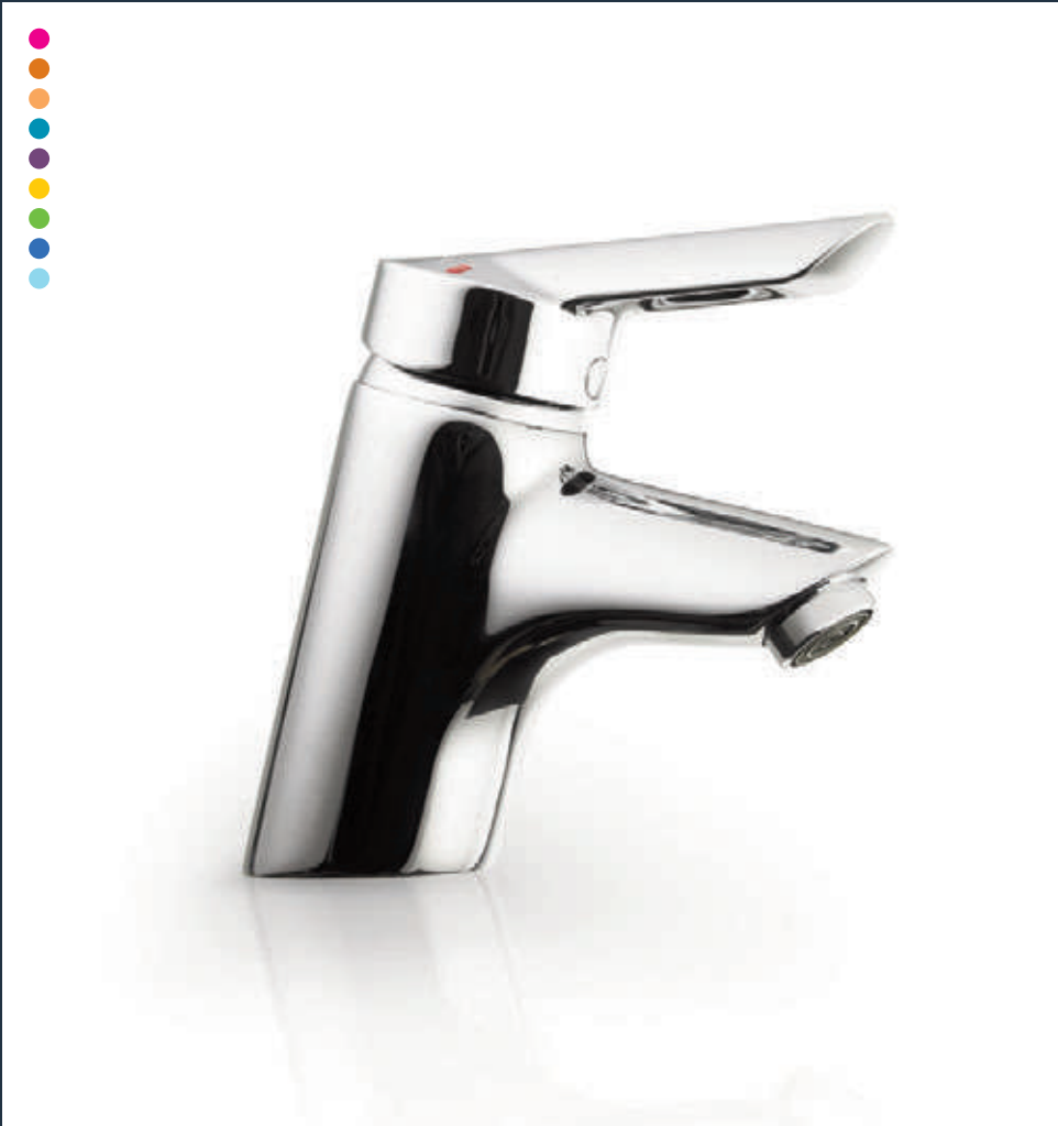
B8260AA Piccolo 21 Single lever monoblock basin mixer, without pop-up waste. This tough and easy to clean design has clear hot/cold identification that will not wear off and a special seal to protect the ceramic disc cartridge from harsh cleaning fluids. Water economy is optimised by CLICK technology. SPX hoses, built in temperature stop and laminar flow design make this a safe and hygienic mixer ( above ).
