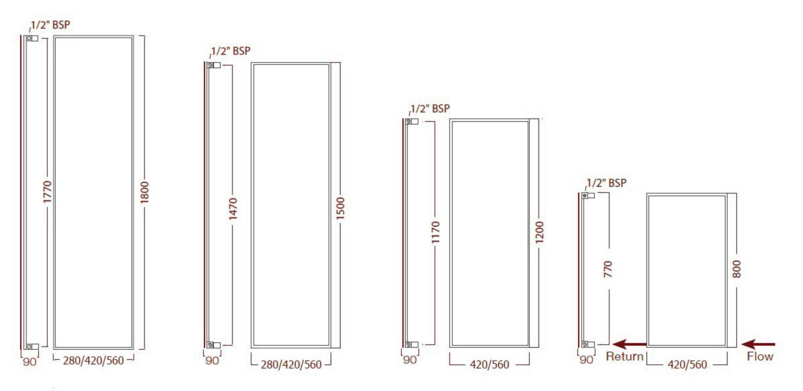
pipe centres = width of radiator + 2 x diameter of angled valve Wall to pipe centres 65mm
