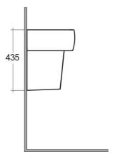
Dimensions: All dimensions in mm tolerance  $\pm 5\%$  for below 200mm and  $\pm 3\%$  for above 200mm. Note: Due to a continuing development programme to improve design and performance, the manufacturer reserves all rights to vary specifications without prior information.
