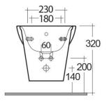
Dimensions: All dimensions in mm tolerance +5% for below 200mm and +3% for above 200mm.
