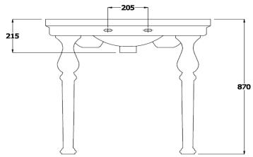
Dimensions: All measurements are in millimeters and are subject to normal manufacturing variations.
