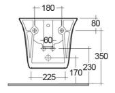
Dimensions: All dimensions in mm tolerance  $\pm 5\%$  for below 200mm and  $\pm 3\%$  for above 200mm. Note: Due to a continuing development programme to improve design and performance, the manufacturer reserves all rights to vary specifications without prior information.
