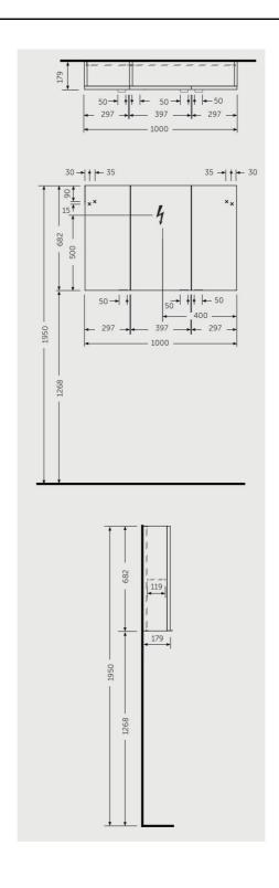
Dimensions: All dimensions in mm tolerance  $\pm 5\%$  for below 200mm and  $\pm 3\%$  for above 200mm. Note: Due to a continuing development programme to improve design and performance, the manufacturer reserves all rights to vary specifications without prior information.
