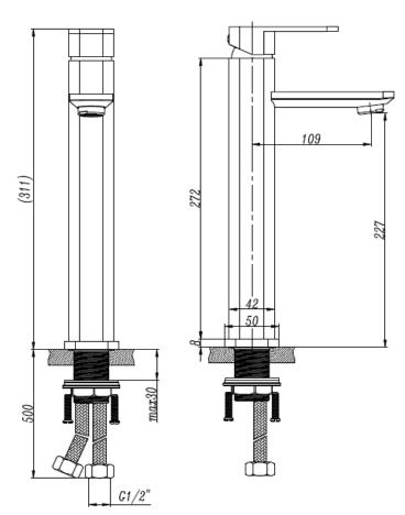
Dimensions: All measurements are in millimeters and are subject to normal manufacturing variations.
