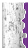
Mershield Stayclear coating creates a smooth layer over the surface of natural glass, lowering surface friction, making it easier for water, soap and lime deposits to run off the glass.
