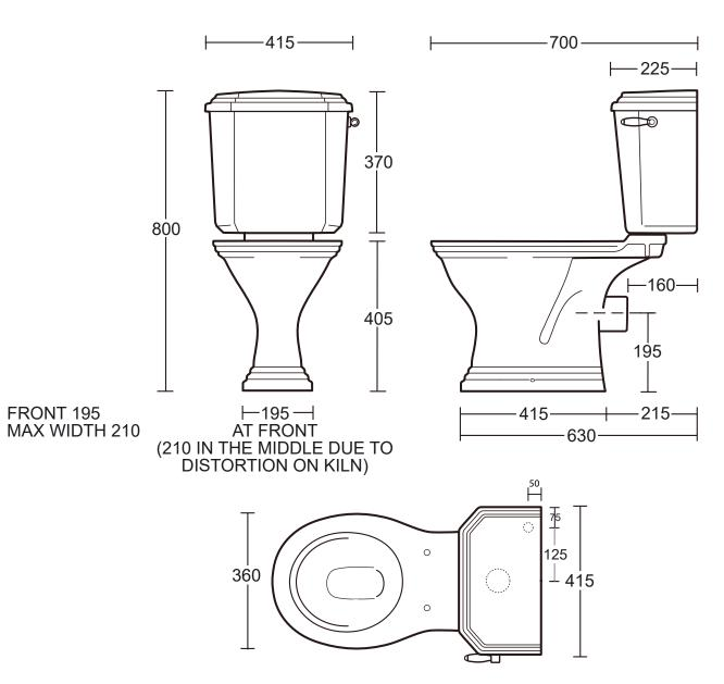
Cistern attached to pan with bolt through fixings (supplied)
