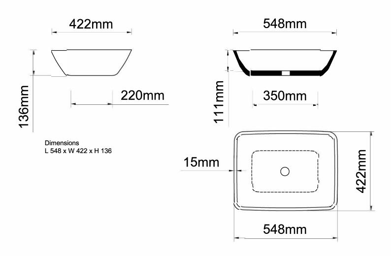
Do not scale from this drawing, only dimensions given should be used. For illustrative purposes only, not for manufacture
