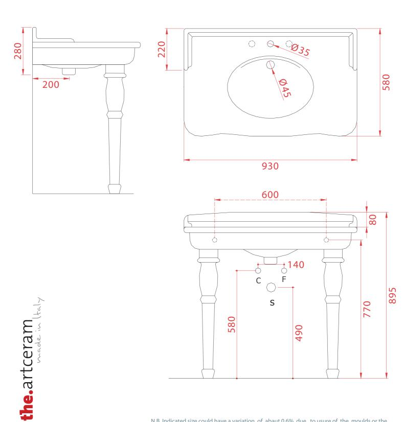
N.B. Indicated size could have a variation of abaut 0,6% due to usure of the moulds or the variations of the materials' technical characteristics used in the mixture.
