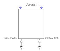
Vertical mount All Dimensions are in mm Max.Working Pressure: 10 Bar Max.Working Temperature: 120° C Inlet / Outlet : 1/2" BSP Fuel : E/H/D
