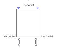
Horizontal mount All Dimensions are in mm Max.Working Pressure: 10 Bar Max.Working Temperature: 120° C Inlet / Outlet : 1/2" BSP Fuel : H
